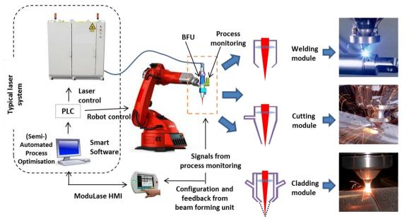
Figure 1 shows a schematic overview of the ModuLase system.
